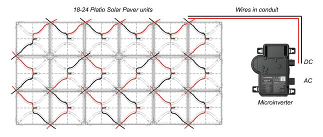
When connecting Platio elements together in series never under any circumstances exceed the SELV (safety extra low voltage) code.
